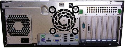
To install the fan, reverse the removal procedure. Be sure to orient the air flow out of the unit.
